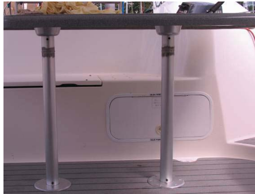
Figure 2.4 Locker under stern cockpit seat with manual bilge pump bilge and pump selector valves
