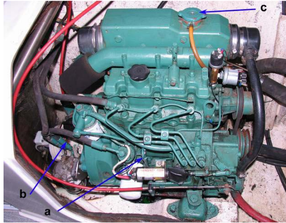
Figure 3.1 Port engine showing positions to check engine oil level (a), gearbox oil level (b) and cooling fluid (c)
