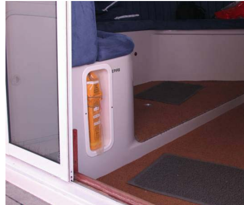
Figure 2.2 EPIRB stowed just inside saloon at cockpit entrance
