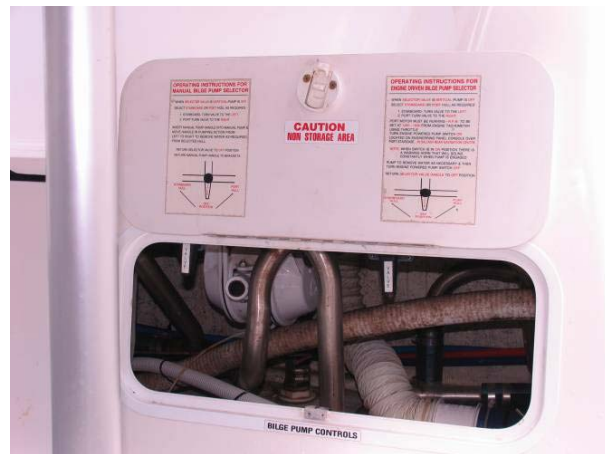
Figure 2.5 Bilge pump valve levers to select port or starboard hulls for hand bilge pump (shown inside locker at back) and mechanical bilge pump.
