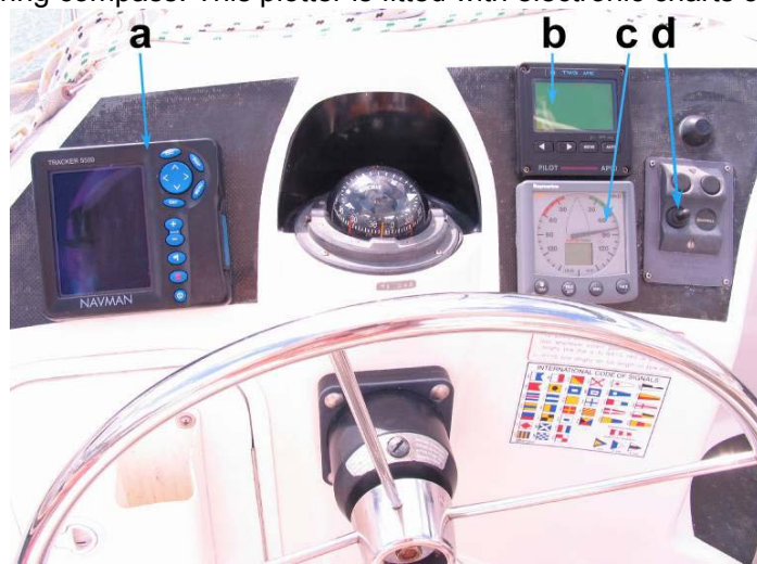
Figure 3.5 Sailing Instruments at helm, showing NavMan GPS chart plotter (a); autopilot control unit with rudder indicator (figure 3.5.b); Raymarine ST60 apparent wind speed and direction indicator (c) and anchor switch assembly (d).
