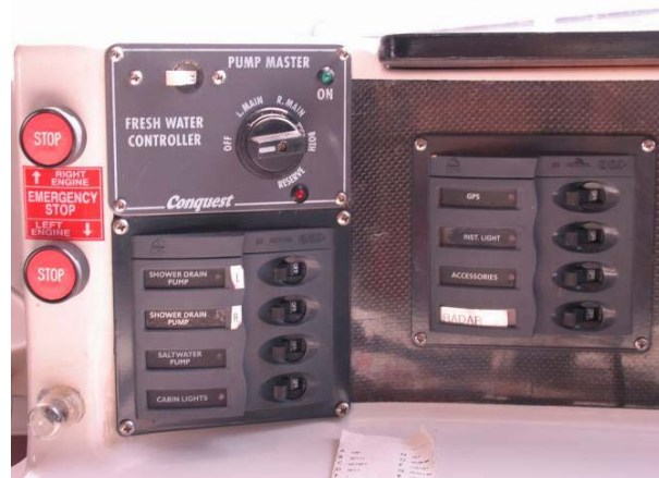
Figure 4.3 Instrument control panel (with circuit breakers) located above the chart table.
